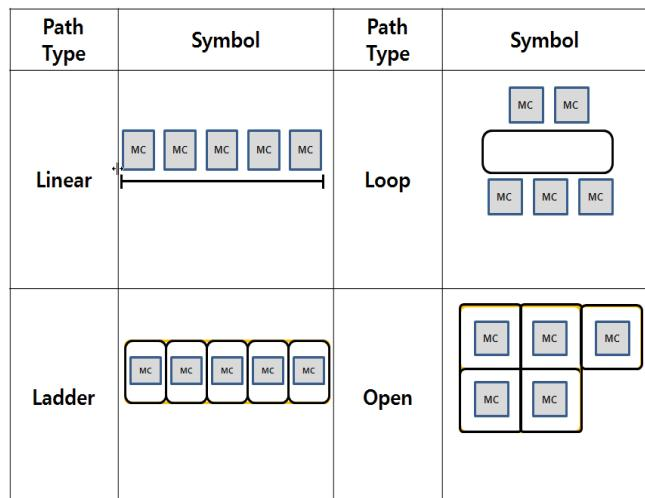
Fig. 3 Transport path type of FMS
