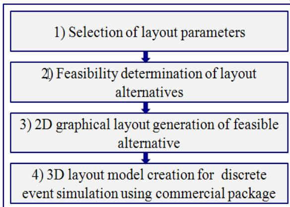
Fig. 5 Proposed procedure for FMS layout design
