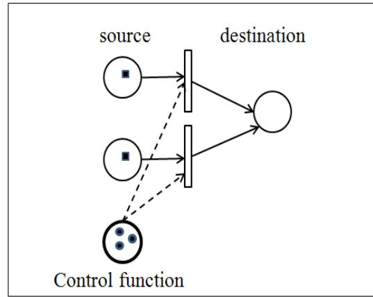
Fig. 18 Supply selection control sub-pattern
