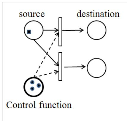
Fig. 16 Destination selection control sub-pattern
