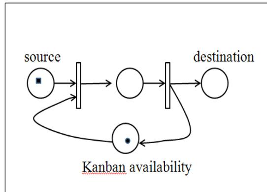
Fig. 17 Work-in-Process control sub-pattern
