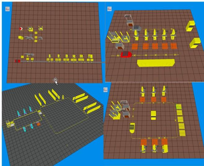
Fig. 12 FMS layout configurations in 3D form
