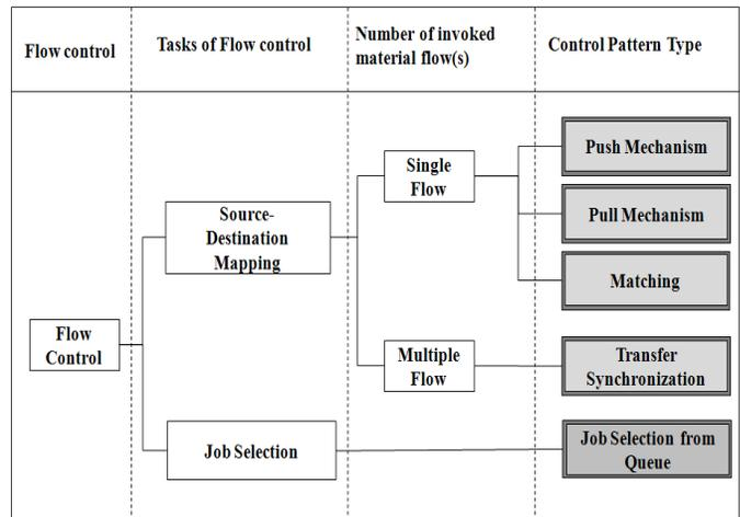
Fig. 13 Tasks of Flow Control
