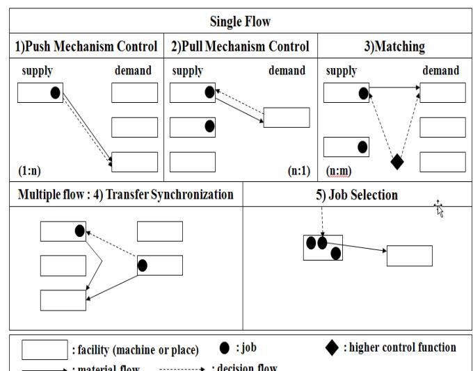
Fig. 14 Control Mechanism of Five Supervisory Control Patterns
