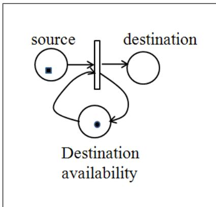
Fig. 15 Blocking avoidance control sub-pattern
