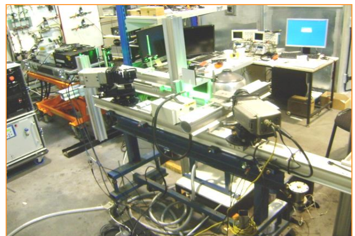
Fig 2: experimental Stereo PIV set-up
