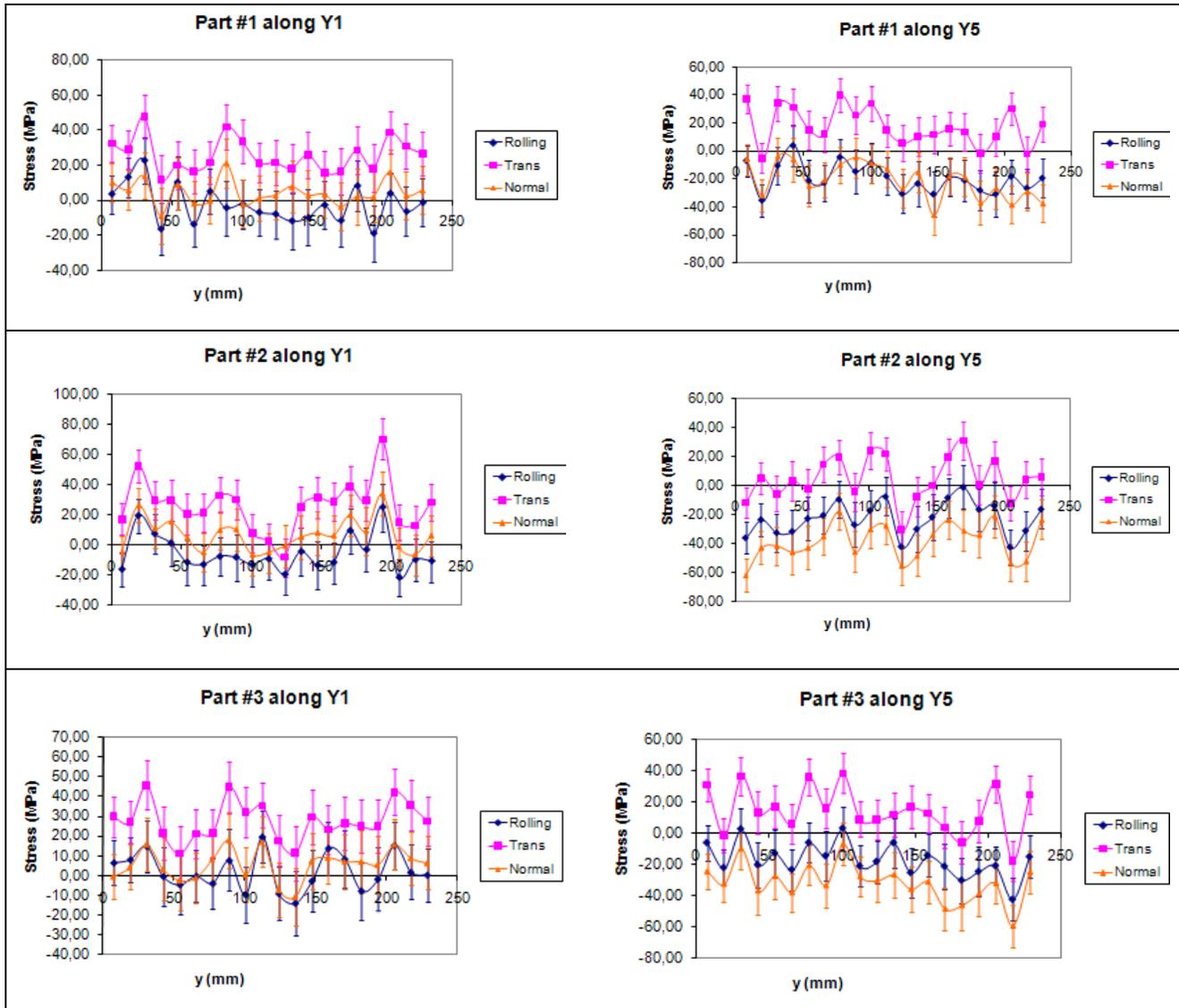
Fig. 7a Rolling, transverse and normal components of residual stress for standard material (parts #1, #2, #3)
