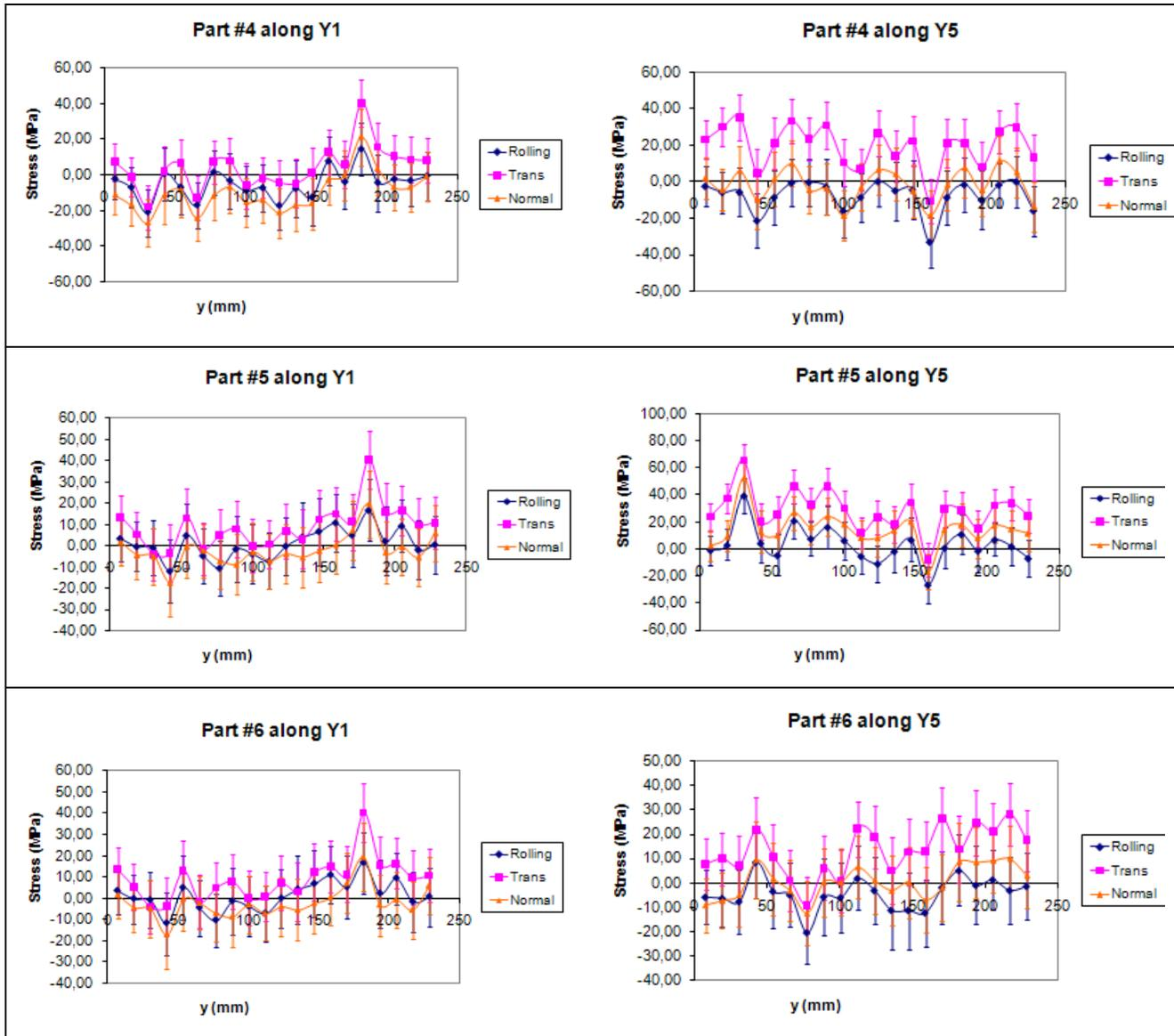
Fig. 7b Rolling, transverse and normal components of residual stress for controlled material (parts #4, #5, #6)
