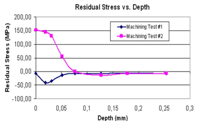
Fig. 4 Stresses induced from machining [1]
