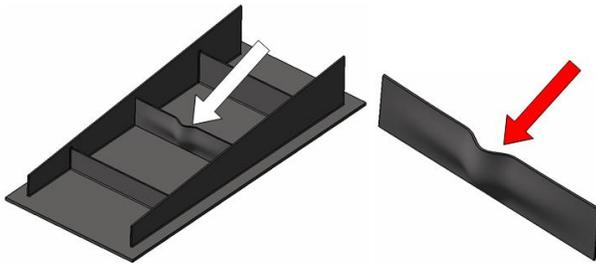
Fig. 1 Oil canning of a thin wall
