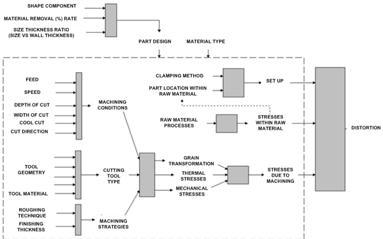
Fig. 2 Source of residual stresses related to the machining of parts
