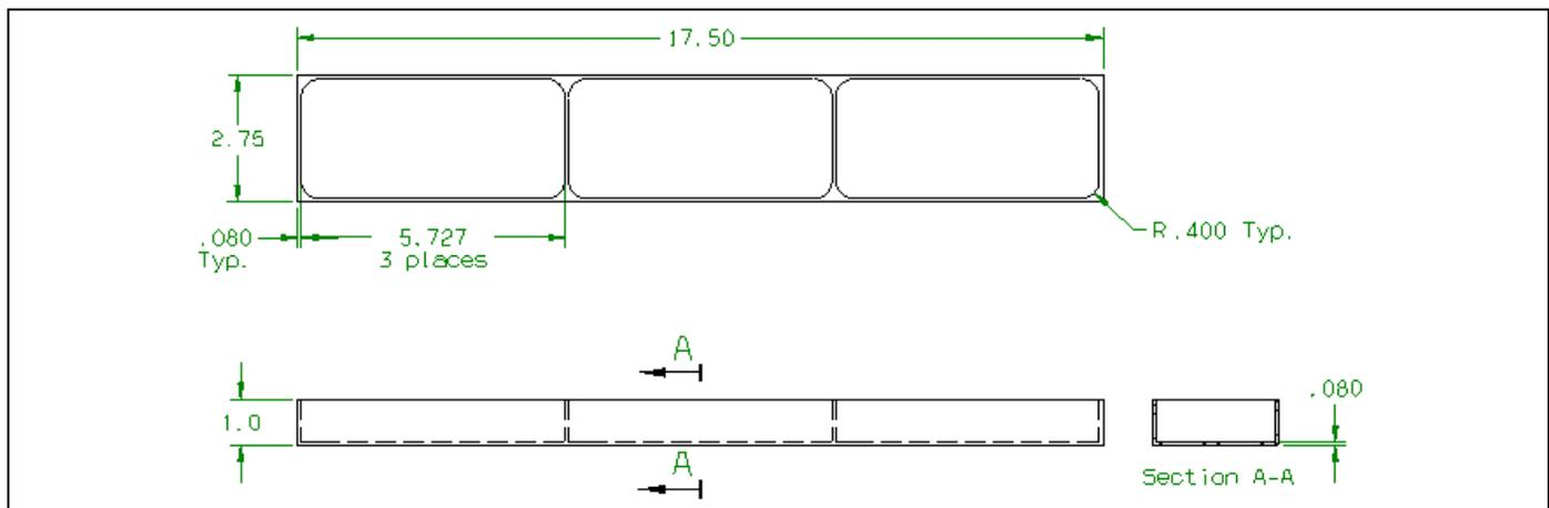
Fig. 5 Part model specifications (dimensions are in inches)
