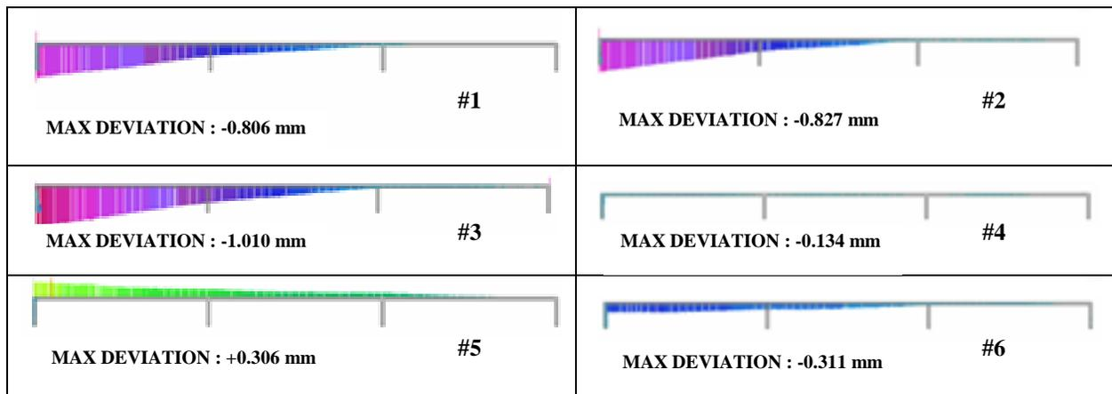
Fig. 9 Longitudinal cross-section of the machined part and representation of the deformation for standard material (#1, #2, #3) and controlled material (#4, #5, #6)
