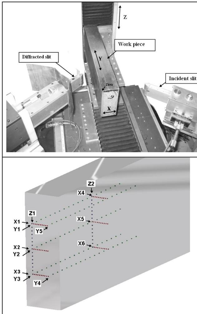
Fig. 6 Location of the stress measurements using the Neutron diffraction method
