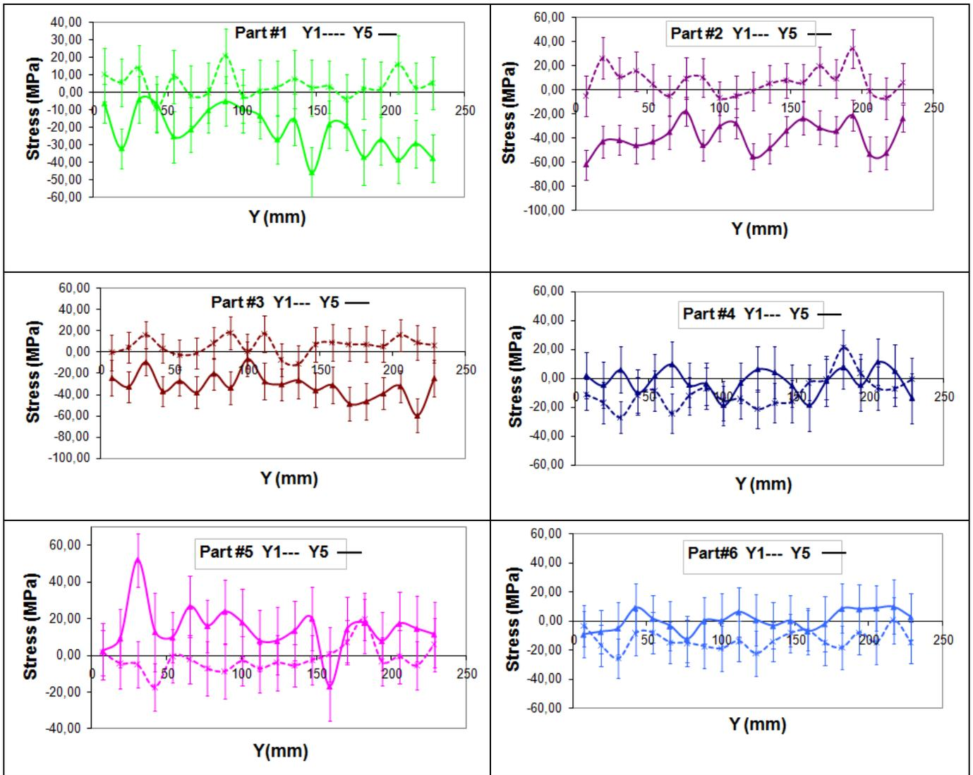
Fig. 8 Focus on normal component (X-axis) of residual stress along longitudinal direction Y1 (bottom) and Y5 (top) for standard material (#1, #2, #3) and controlled material (#4, #5, #6).
