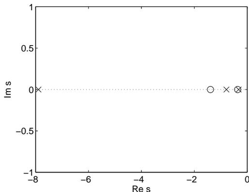
Fig. 6. Pole-zero map of system  $G_7(s)$  in Example 7.
