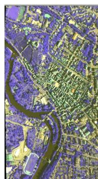
Fig5. Example of digital orthophoto resulted from orthorectification of digital photogrammetric camera image using Lidar DSM.
