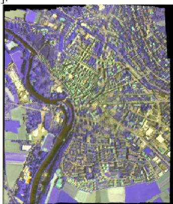
Fig.6 Mosaic of digital orthophotos that resulted from orthorectification of digital photogrammetric camera images using Lidar DSM .
