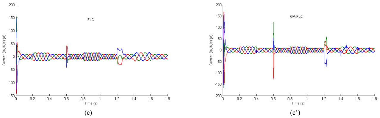
Fig. 11 three phase stator current: (c) FLC (c') FLC-GA.
