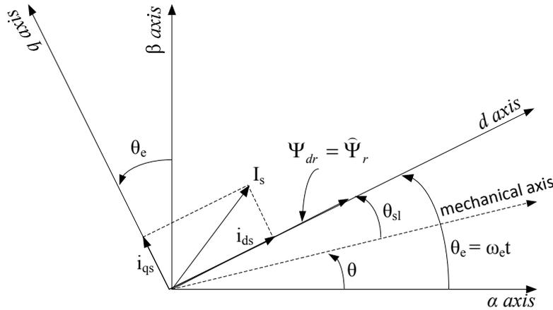
Fig. 1 vector diagram for indirect field oriented control
