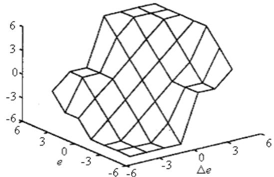
Fig. 4 control surface for the conventional fuzzy controller.
