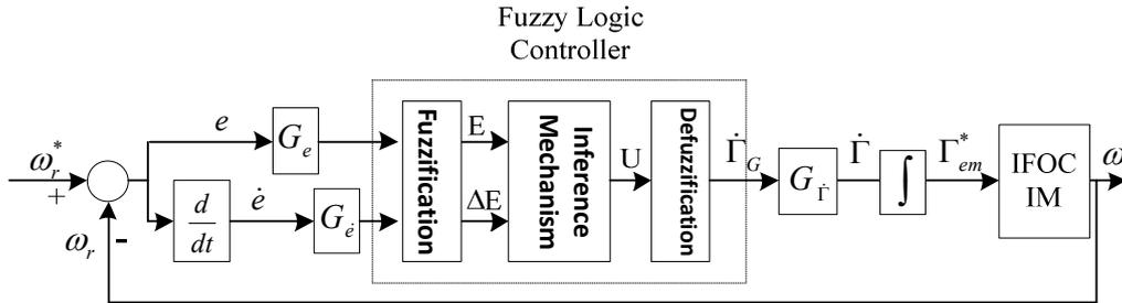
Fig. 2 basic structure of the fuzzy logic controller for indirect field oriented control.
