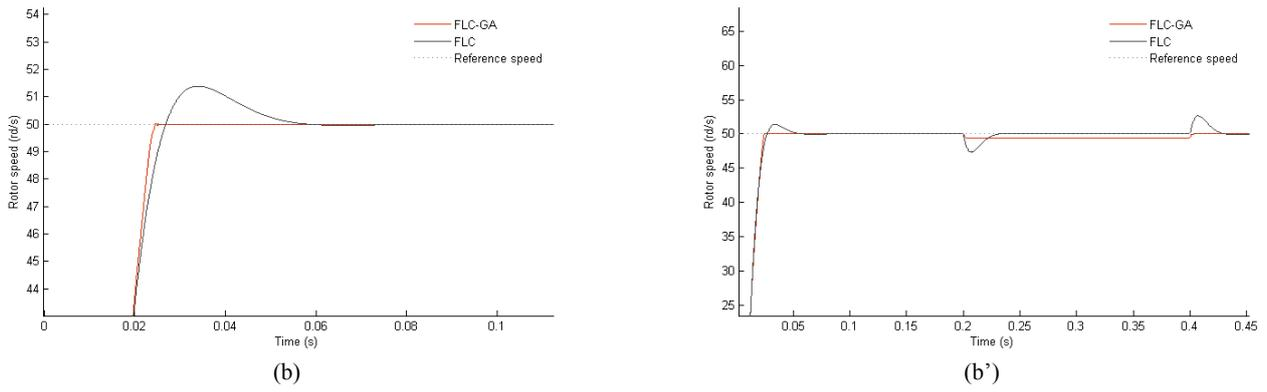
Fig. 10 zoom speed: (b) starting transient performance and overshoot (b') response due to load and unload change.
