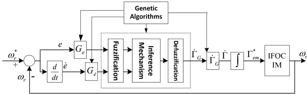
Fig. 7 basic structure of the genetic algorithms based fuzzy logic controller for indirect field oriented control.
