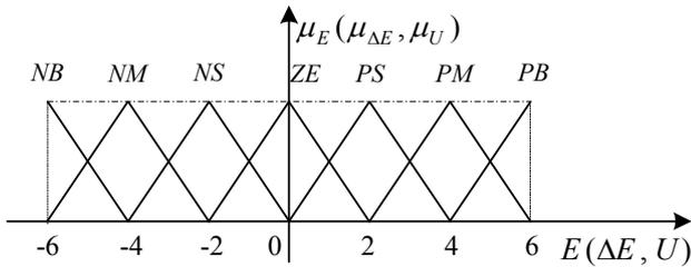
Fig. 3 the shape of membership functions for fuzzy logic controller.
