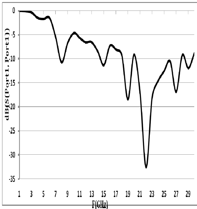
Fig: 15 Return Loss Vs Frequency of Modified Circular patch with Microstrip feed at position 2. R=15mm, h=1.6mm, resonant frequency=22GHz.
