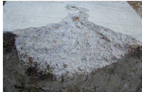
Fig. 11 expansion anchor subjected to shear
