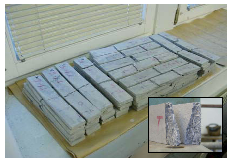
Fig. 2 failed test specimens – material (i)
