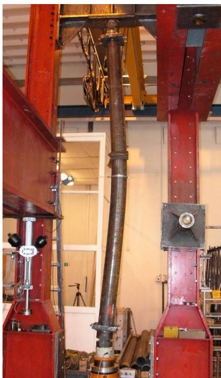
Fig. 13 steel-concrete column composed of high-strength materials subjected to compression
