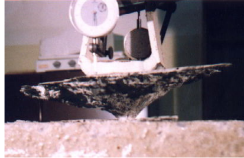
Fig. 10 expansion anchor subjected to tension
