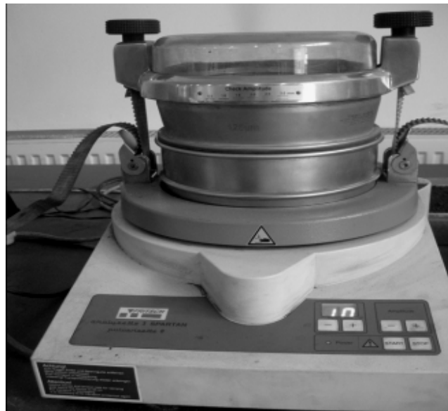
Fig.9 Apparatus for waste classification
