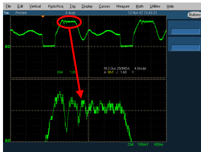
Fig. 3 Disturbances in terminals of the Drain-Source V_{DS} of the power MOSFET.
