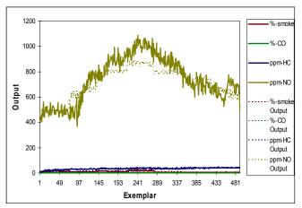
Figure 10. Desired Output and Actual Network Output
