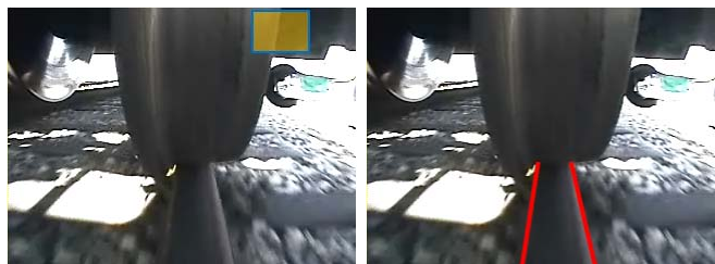
(a) template for detecting the wheels (b) line component of the rail
