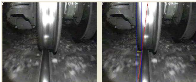
Fig.11 experimental results of the relative displacement measurement based on real-time image processing method
