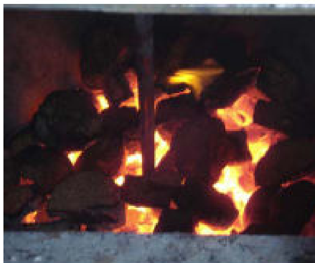
Fig. 5: a view of combustion zone in the gasifier
