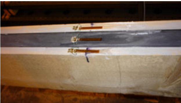
Fig. 15 strain gauges on bottom edge of timber beam and on CFRP
