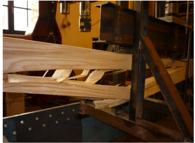
Fig. 17 failure of CFRP strengthened timber beam – timber failure
