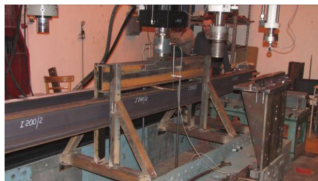
Fig. 4 test arrangement and realization – steel beams with CFRP
