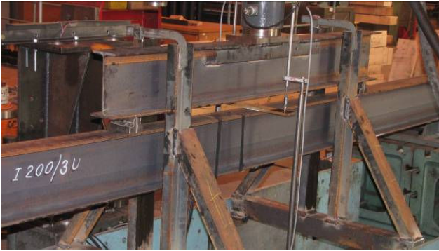
Fig. 5 test realization – steel beams with CFRP: load introducing to the specimen through the stiff girder
