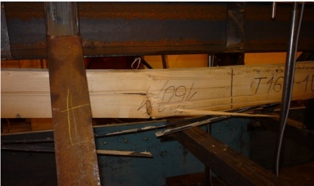
Fig. 16 failure of CFRP strengthened timber beam – lamella rupture
