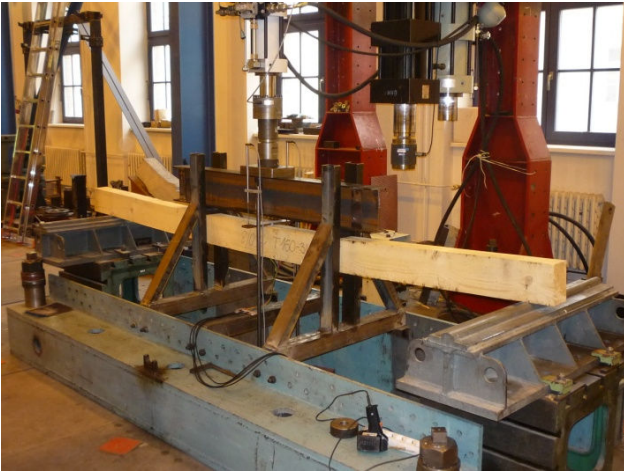
Fig. 14 test arrangement and realization – timber beams with CFRP
