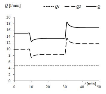
Fig. 14 Simulation model of P controller – time dependencies of action signal  $Q_2(t)$ ,  $Q_1(t)$  and Q(t)
