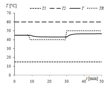
Fig. 13 Simulation model of P controller – time dependencies of  $T_1(t)$ ,  $T_2(t)$ ,  $T_R(t)$  and T(t)
