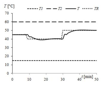
Fig. 15 Simulation model of PID controller – time dependencies of  $T_1(t)$ ,  $T_2(t)$ ,  $T_R(t)$  and T(t)
