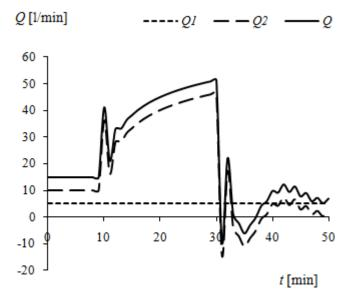
Fig. 18 Simulation model of PID controller – time dependencies of action signal  $Q_2(t)$ ,  $Q_1(t)$  and Q(t) of non-controlable system
