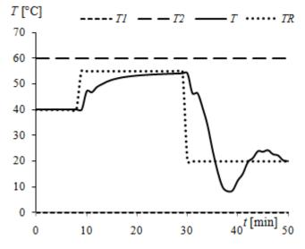
Fig. 17 Simulation model of PID controller – time dependencies of  $T_1(t)$ ,  $T_2(t)$ ,  $T_R(t)$  and T(t) of non-controllable system
