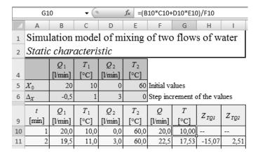
Fig. 6 Simulation model of static characteristics in MS Excel table
