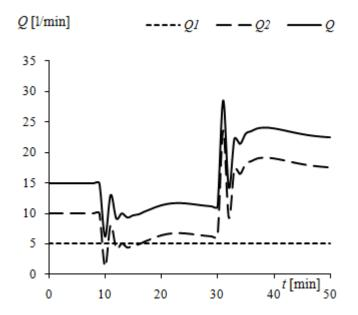
Fig. 16 Simulation model of PID controller – time dependencies of action signal  $Q_2(t)$ ,  $Q_1(t)$  and Q(t)
