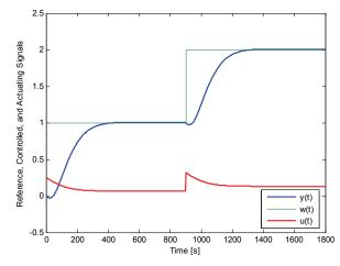
Fig. 6 control of plant using continuous-time controller - simulation
