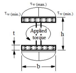
*Figure 6.* Cross-sectional of a beam with illustrated maximum warping stress.
