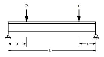
Figure 1. Beam and loading
