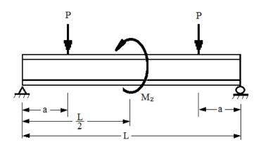
Figure 2. Combined Bending and Applied Torsion
