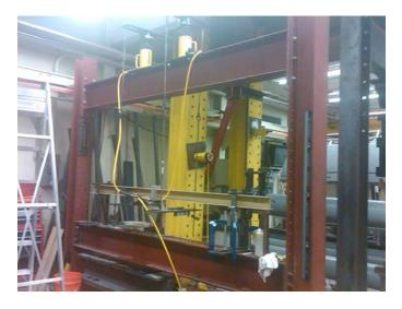
*Figure 3.* Experimental test setup used for a series of FRP beams
