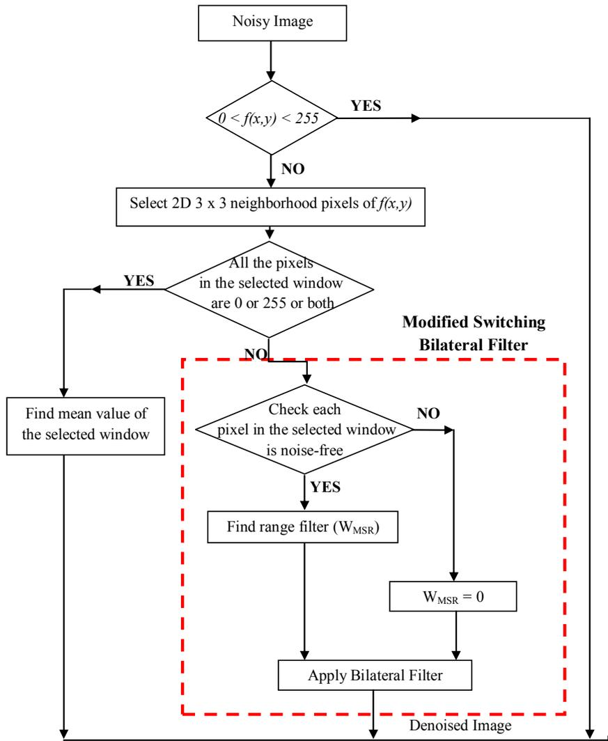
Fig. 2. Flowchart of modified switching bilateral filter
