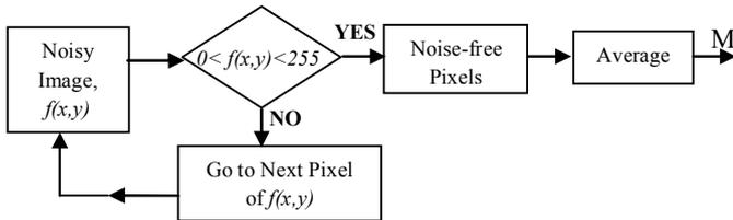
Fig. 1 Block diagram of computation of global trimmed mean value
