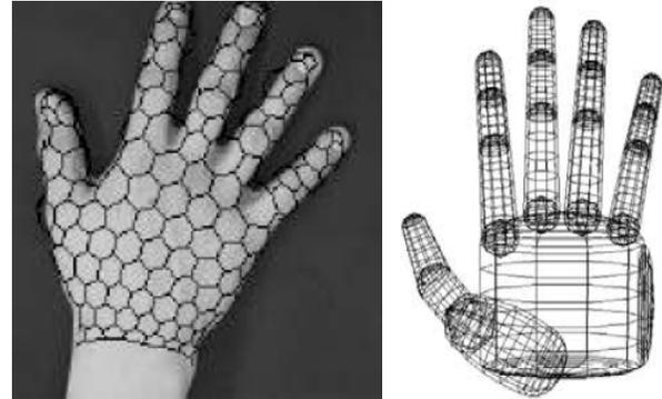
Fig.2 a) Hand tracking using 3D Point Distribution Model from [8] and b) Quadrics-based hand model from [9]
