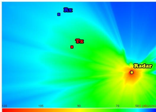
Fig. 18 Field strength distribution around radar
