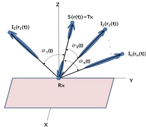
Fig. 4 Geometry of Tx-Rx and multiple interferers
