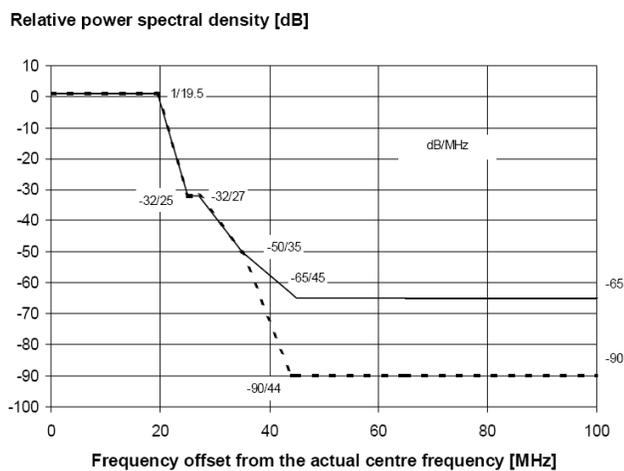
Fig. 19 Tx spectrum mask and receiver selectivity
