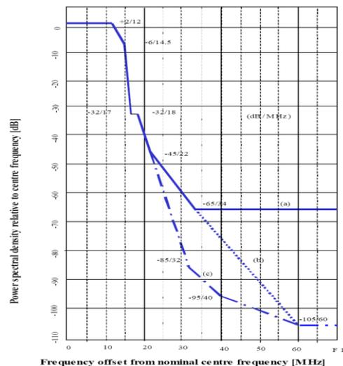
Fig. 8 Tx spectrum mask and receiver selectivity
