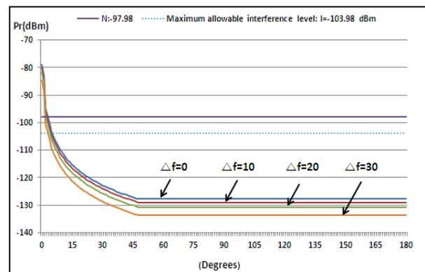
Fig. 21 Received interference power for azimuth angle
