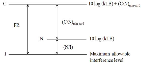
Fig. 3 Concept of protection ratio
