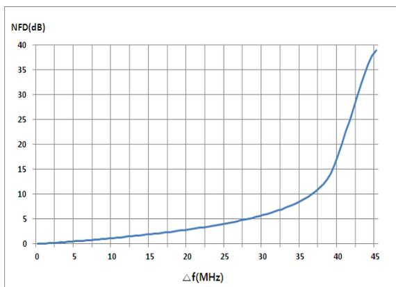
Fig. 20 Calculated  $NFD$  with frequency offset
