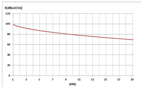
Fig. 6 Field strength values between Tx and Rx
