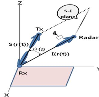
Fig. 2 Geometry of Tx, Rx and radar systems
