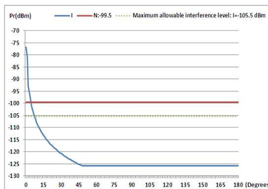
Fig. 13 Interference power of Rx in azimuth angle
