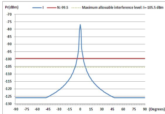
Fig. 14 Interference power of Rx in elevation angle
