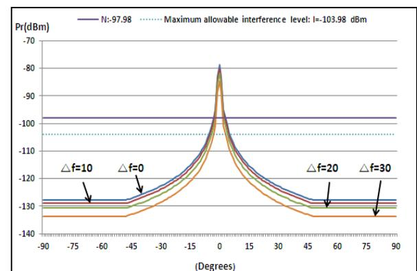
Fig. 22 Received interference power for elevation angle
