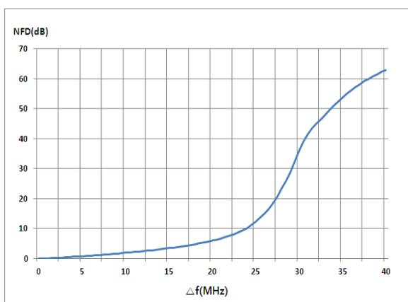
Fig. 10 Calculated  $NFD$  with frequency offset
