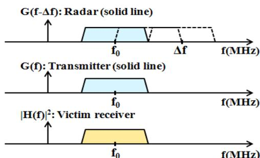
Fig. 9 Frequency allocations of FWS and radar
