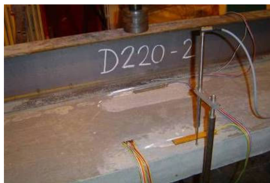
Fig. 7 detail of strain gauges on concrete slab
