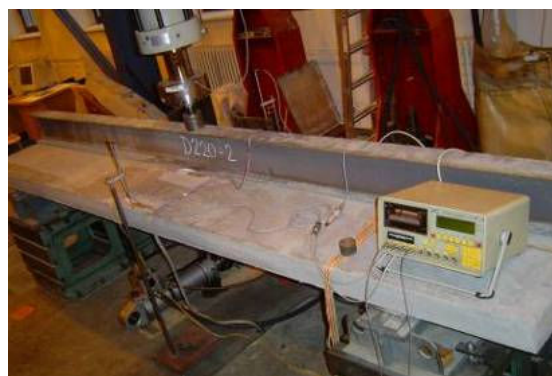
Fig. 5 illustration of test set-up, specimen and measuring apparatus
