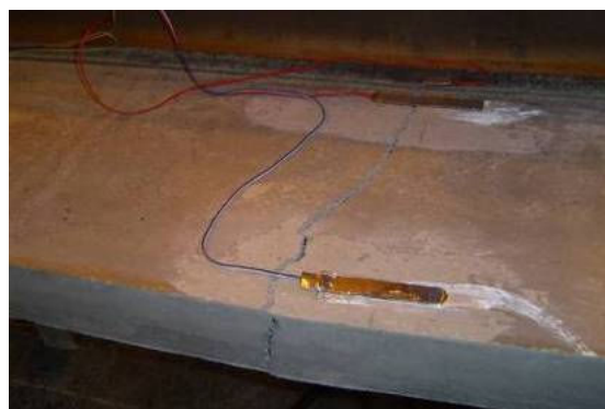
Fig. 7 detail of strain gauges on concrete slab
