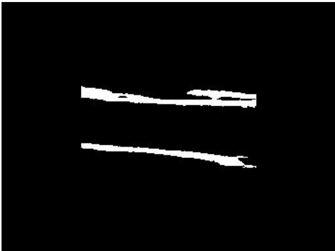
Fig. 7: Ultrasound image after removing parts smaller than 600 pixels
