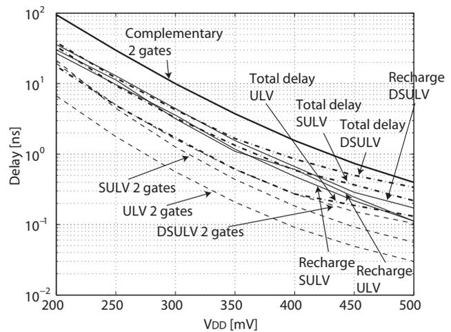
Fig. 11. Recharge delay, the delay through two ULV gates and total delay through an ULV latch and two ULV gates.
