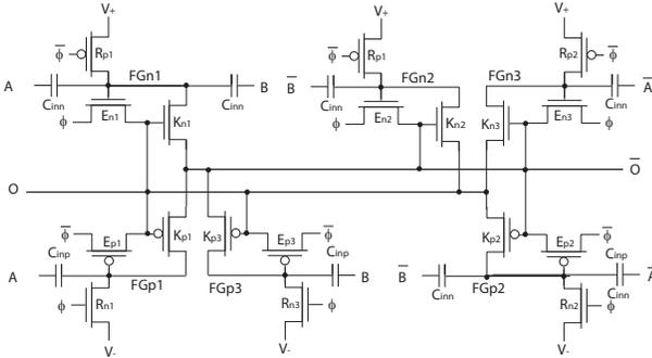
Fig. 8. Differential ULV NAND (N2) gate.
