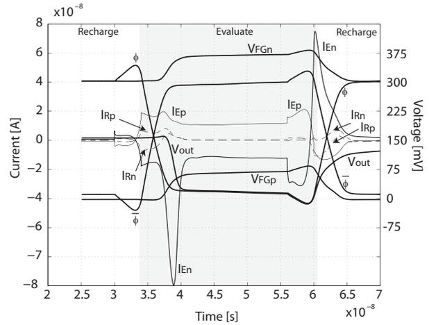
Fig. 4. The response of the ULV inverter. The supply voltage is  $300mV$
