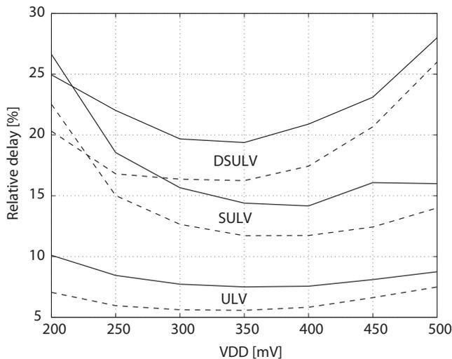
Fig. 13. The relative delay through 2 inverters for different supply voltages. Solid lines represents relative delay assuming ideal clock signals and the dashed lines represents the relative delay assuming normal (Norm) clock drivers.
