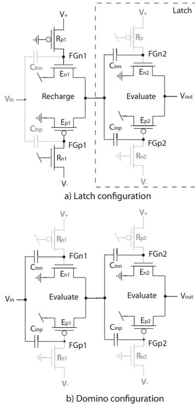
Fig. 3. Simple ULV Inverter, a) latch configuration and b) domino configuration.
