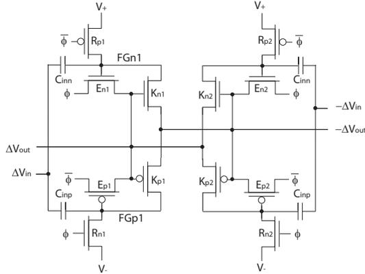
Fig. 5. Differential ULV inverter (DSULV).
