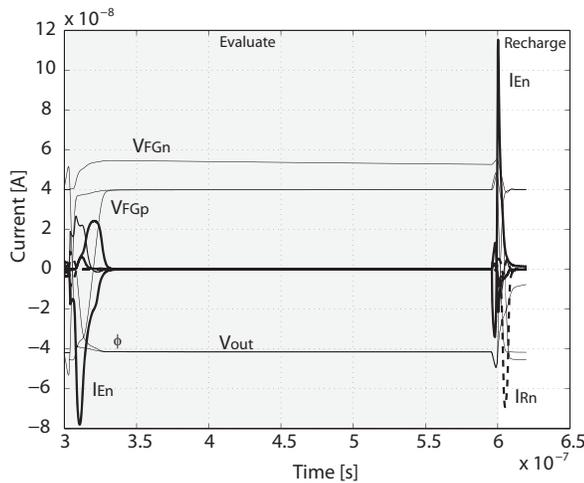
Fig. 10. The response of the DSULV inverter. The supply voltage is 300mV.
