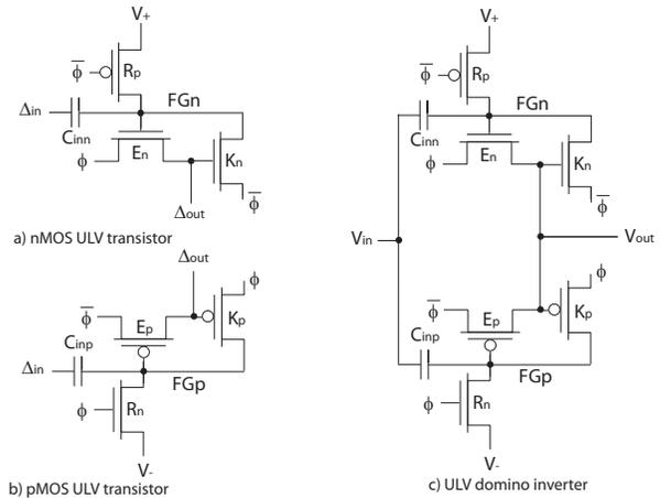
Fig. 1. a) *nMOS ULV transistor*, b) *pMOS ULV transistor* and c) *static ultra low-voltage semi-floating-gate recharge inverter*. The transistors labeled  $K_n$  and  $K_p$  provide a feedback making the output static.
