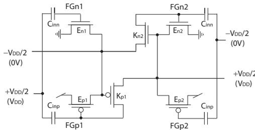
Fig. 6. Differential ULV inverter in evaluate mode assuming an input  $\Delta V_{in} = V_{DD}/2$ .
