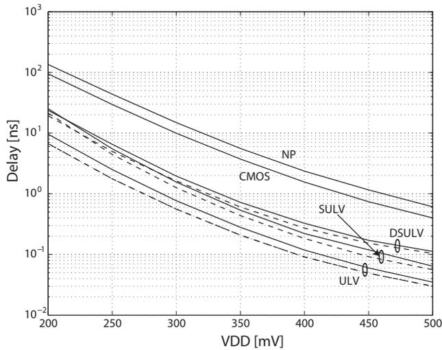
Fig. 12. The delay through 2 inverters for different supply voltages.
