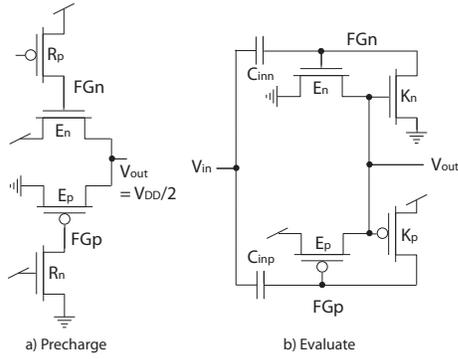
Fig. 2. a) ULV inverter in precharge mode and b) ULV inverter in evaluate mode.
