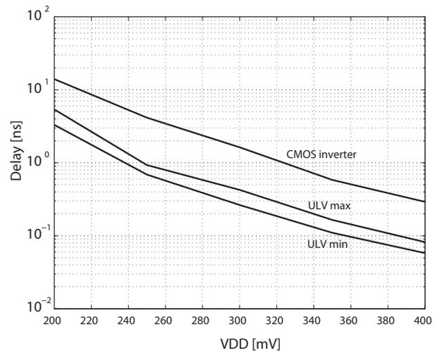
Fig. 9. Maximum and minimum delay for the ULV differential NAND2 gate.
