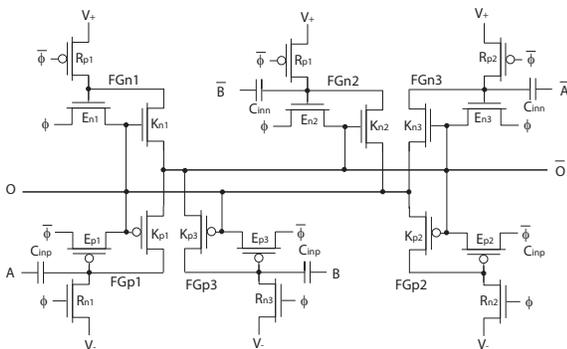
Fig. 7. Differential ULV NAND gate (N1).
