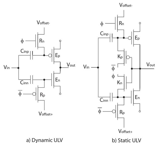
Fig. 1. a) simple ULV inverter and b) static ULV domino logic inverter.
