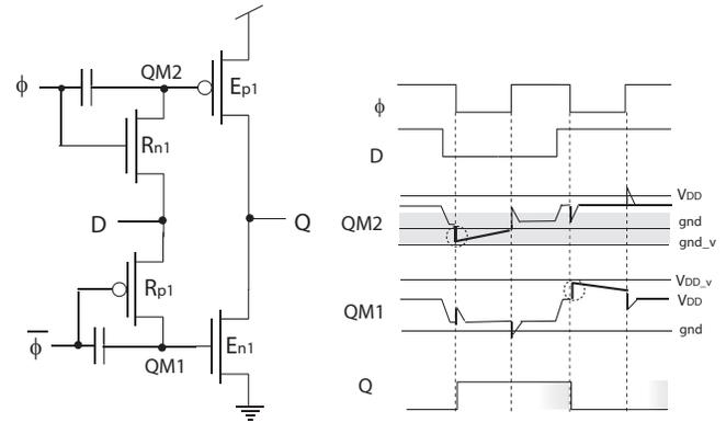
Fig. 5. Dynamic ULV inverting Flip-Flop .
