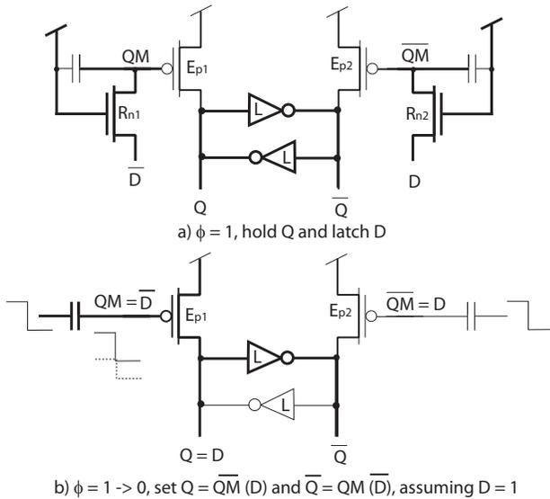
Fig. 8. The single phase high-speed ULV Flip-Flop.
