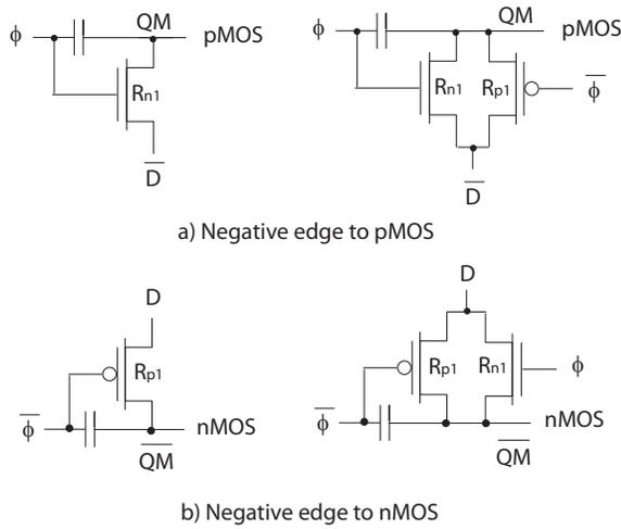
Fig. 3. Dynamic ultra low-voltage high speed master latches.
