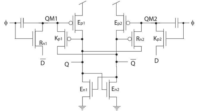
Fig. 6. Low power single phase differential dynamic ULV Flip-Flop.
