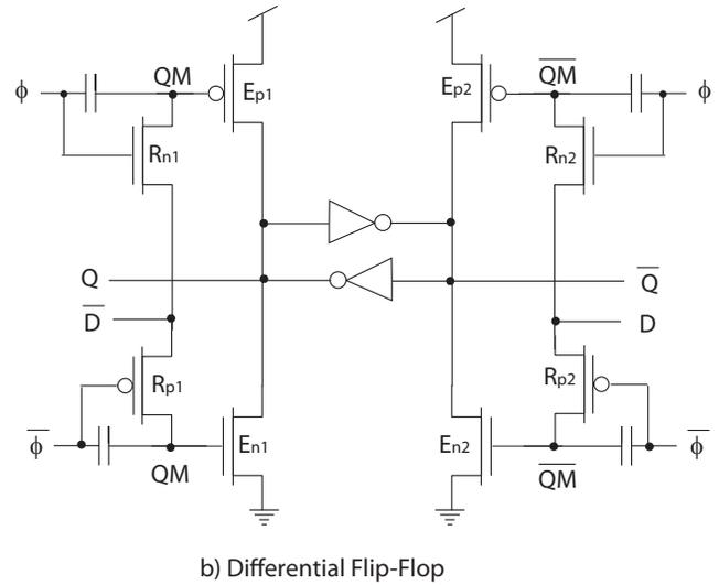
Fig. 9. The symmetric high-speed ULV Flip-Flop.
