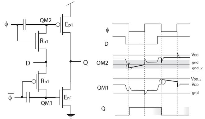
Fig. 5. Dynamic ULV inverting Flip-Flop .
