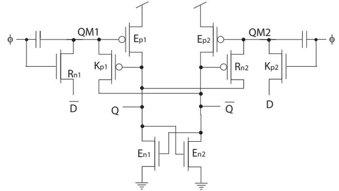
Fig. 6. Low power single phase differential dynamic ULV Flip-Flop.
