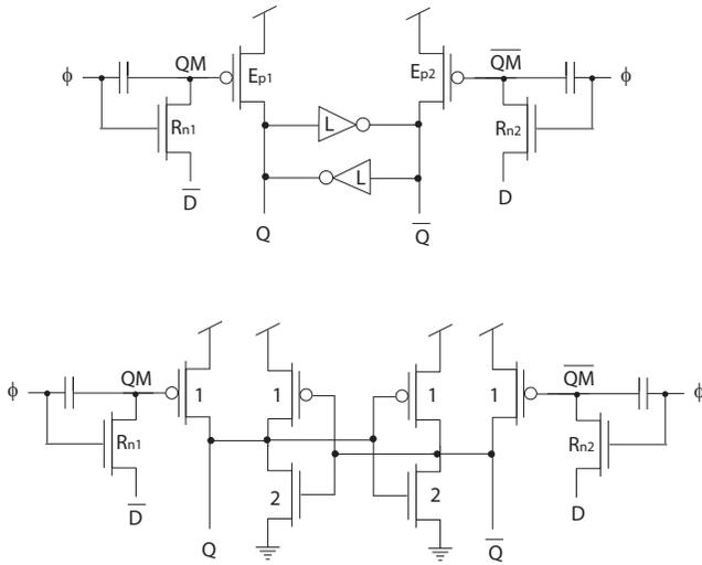
Fig. 7. The single phase high-speed ULV Flip-Flop.
