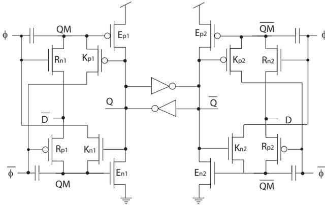
Fig. 10. The low-power symmetric high-speed static ULV Flip-Flop.
