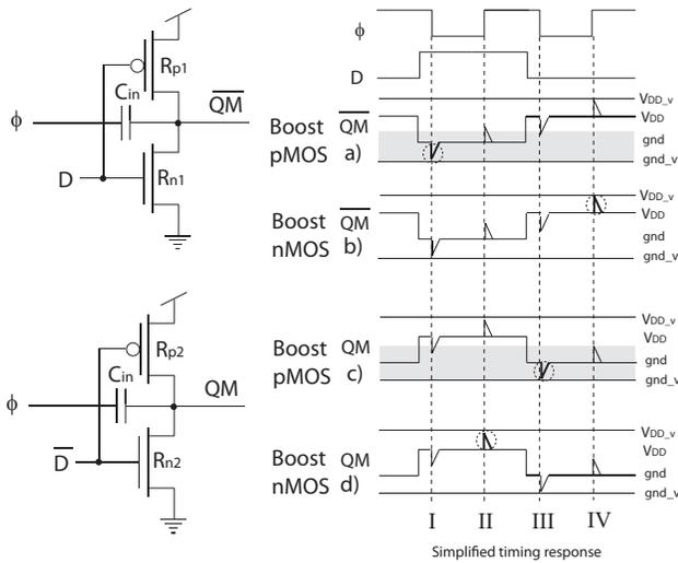
Fig. 2. Ultra Low-Voltage dynamic differential Master latch.
