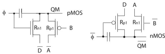
Fig. 4. Quasi static ultra low-voltage high speed master latch.
