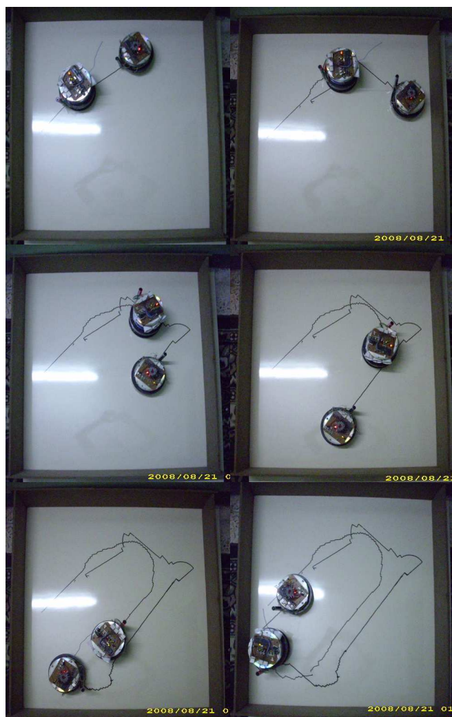
Fig. 15: target and chaser paths during a test for the follow behavior
