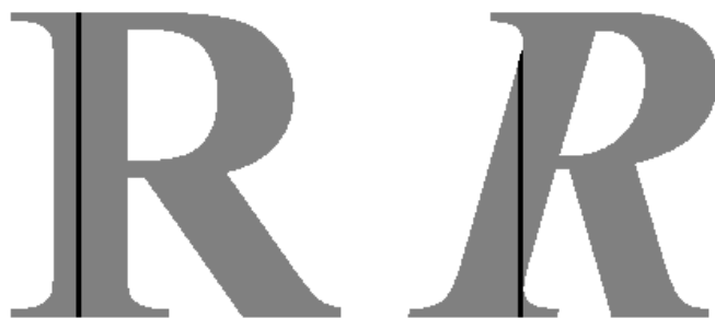
Fig. 17 the longest vertical line of black pixels in the case of a regular letter (left) compared to the longest line for an italic letter (right)
