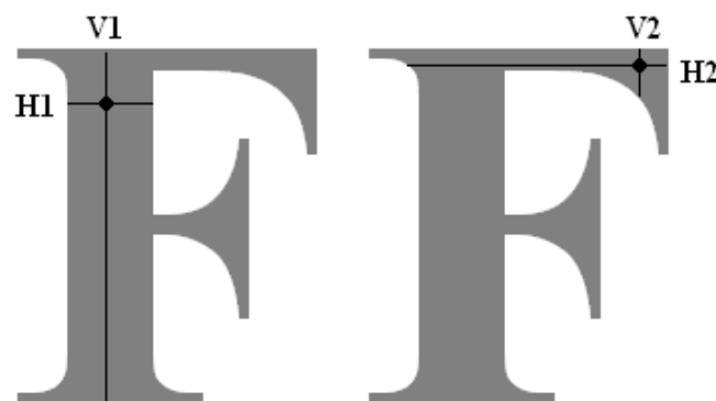
Fig. 15 for the pixel at the intersection of V1 and H1 the dominant will be vertical (V1), while for the pixel at the intersection of V2 and H2 the dominant will be horizontal (H2)
